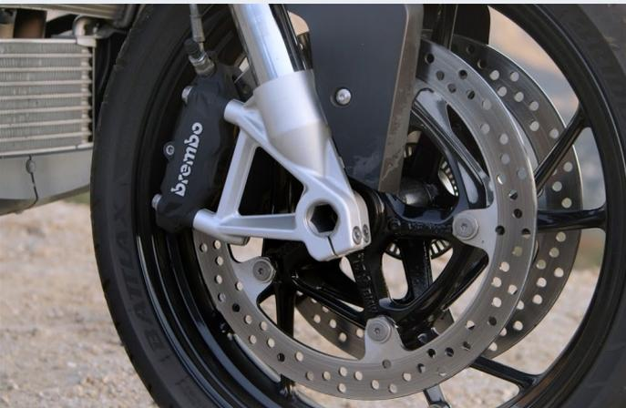
What's happening is that the computer detects that the front wheel is not turning and perceives it to be locked and skidding. In that case weight would be thrown forward off the rear wheel, which would lock easily, de-stabilising the bike which would have two skidding tyres. Hence the minimal braking force applied to the back wheel. On the road, the electronics constantly compare the speed of both wheels and apply the two brakes in the most efficient manner to stop quickly.
